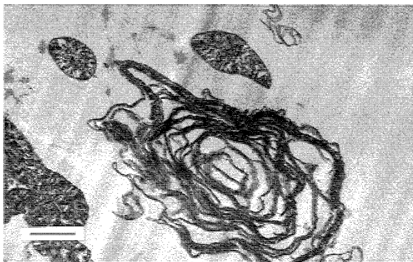
Fig. 2. Electron micrograph of acacia-gelatin-microencapsulated DPPC liposomes by fixation and thin section technique. Bar = 1 \mu\text{m} .
